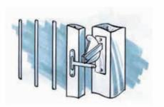
Firstly, position the 'D' latch on the post with tek screws so it will be aligned with the striker bar when the gate is closed. Then fix the striker bar to the vertical gate frame and check for smooth operation.
